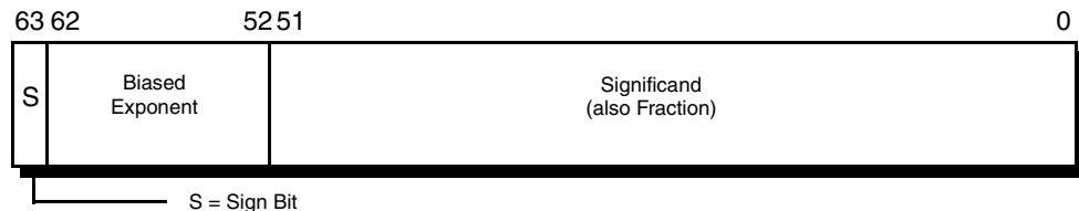
Figure 4-15. 128-Bit Media Floating-Point Data Types
